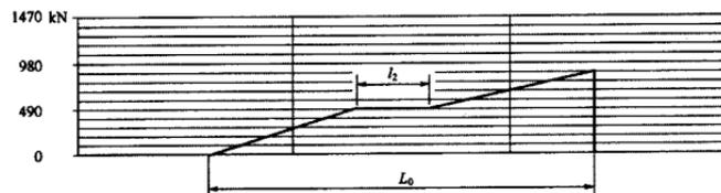
图 A.17 不合格曲线(中间平直线长  $l_2/L_0 > 10\%$ )
